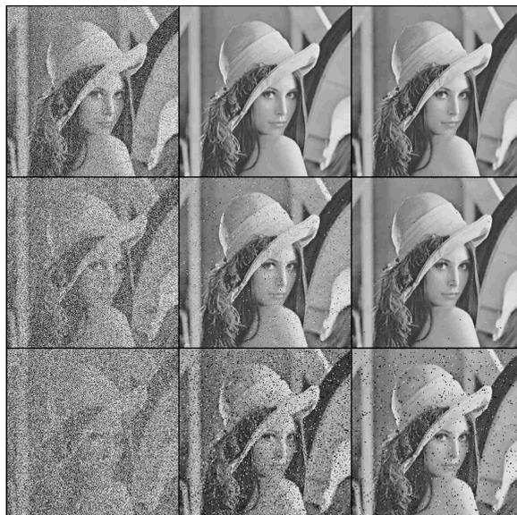
**Fig. 2.** From left to right, first row: An image with 20% of impulsive noise, opening morphological filtering ( $\gamma_A$ ) and opening-closing ( $\varphi_A \gamma_A$ ), second row: image with 50% of impulsive noise, morphological filtering  $\gamma_A$  and  $\varphi_A \gamma_A$ , third row: image with 70% of impulsive noise, morphological filtering  $\gamma_A$  and  $\varphi_A \gamma_A$
